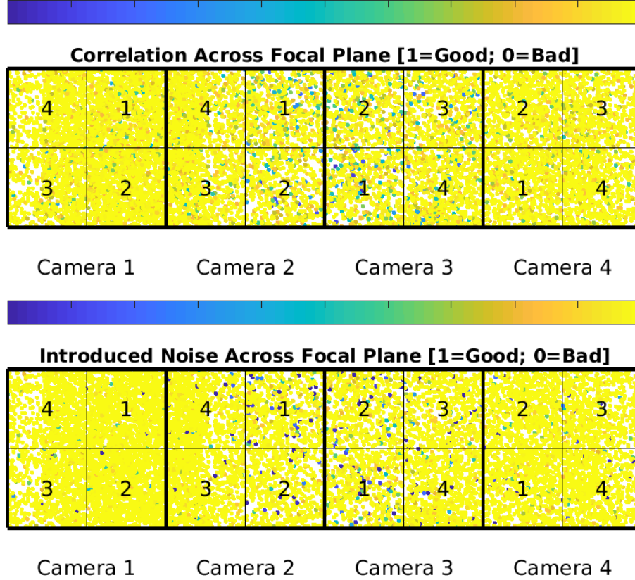
Figure 5: PDC residual correlation goodness metric (top panel) and PDC introduced noise goodness metric (bottom panel) for the two-minute cadence data. The metric values are shown on a focal plane map indicating the camera and CCD location of each target. The correlation goodness metric is calibrated such that a value greater than 0.8 means there is less than 10% mean absolute correlation between the target under study and all other targets on the CCD. The introduced noise metric is calibrated such that a value greater than 0.8 means the power in broad-band introduced noise is below the level of uncertainties in the flux values.
